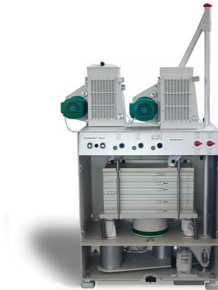
Figure 1. Brabender ® Quadrumat® Senior laboratory mill
