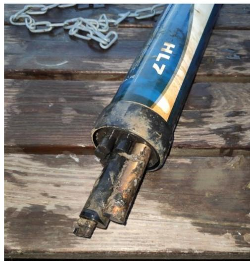
Fig. 4 Applied HYDROLAB- HL 7 multiparameter probe without coverguard
