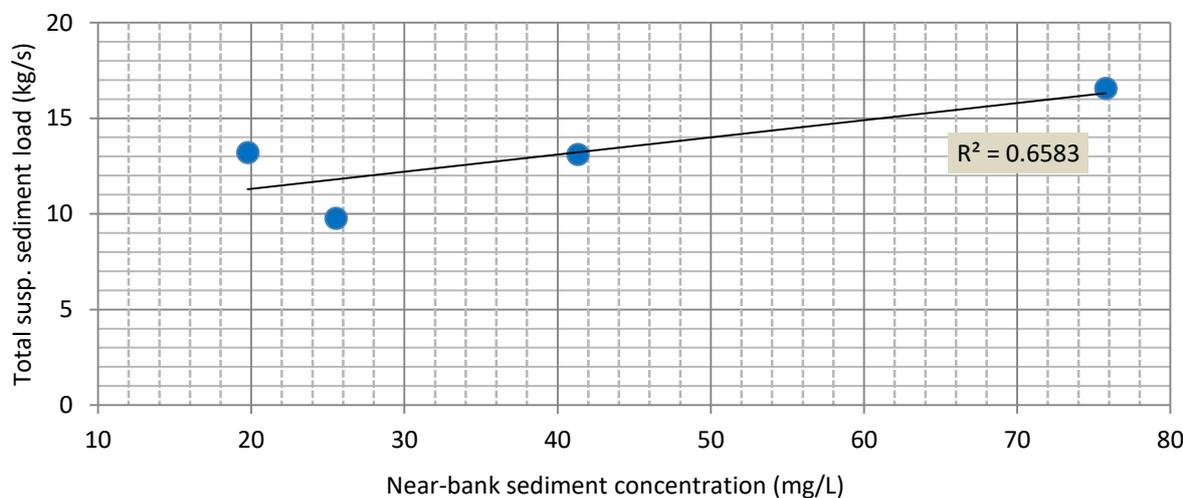
Fig. 9 Suspended sediment yields (kg/s) as a function of near-bank suspended sediment concentration (mg/l)
