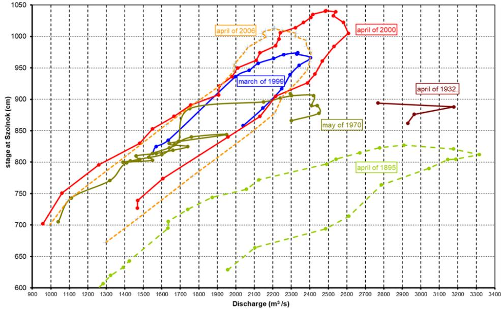
Fig.1 Water level – discharge loop-like curves at Szolnok gauging station (after Kovács and Váriné Szöllösi, 2003)
