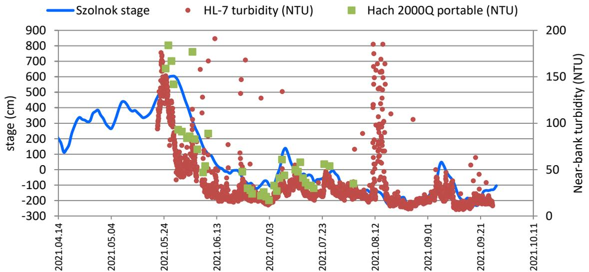
Fig.7 Near-bank turbidity (NTU) and stage (cm) time series at Szolnok
