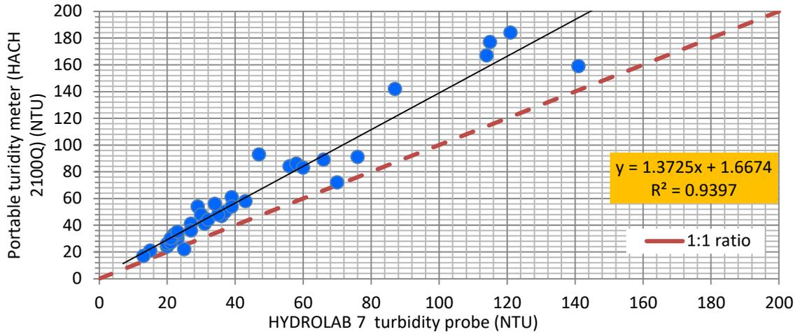
Fig.6 The relationship between the data of the HL 7 probe and portable hand-held turbidity meter (in NTU)
