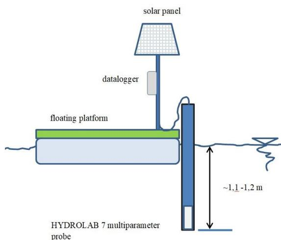
Fig. 5 Design of an installed turbidity measuring probe
