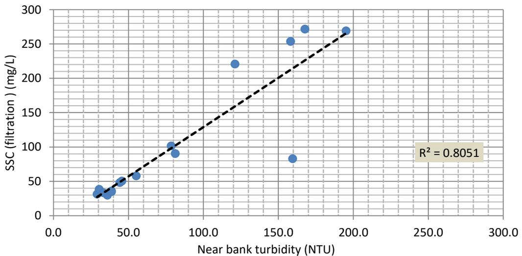
Fig.8 Correlation between the near-bank turbidity (NTU) and suspended sediment concentration (mg/l)
