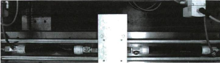
Fig. 5. Mounting PAMs into shorter places than their initial lengths
