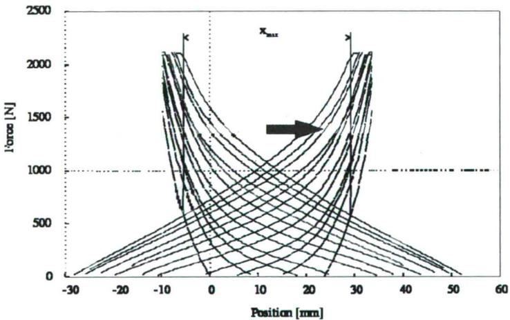
Fig. 6. Extended operation range of PAMs
