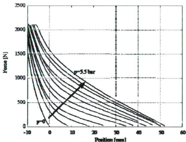
*Fig. 3.* PAM isobaric force-position characteristics
