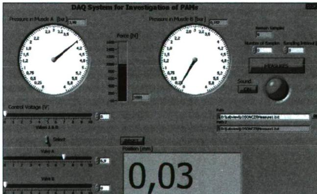
**Fig. 2. Front panel of the LabVIEW program**
