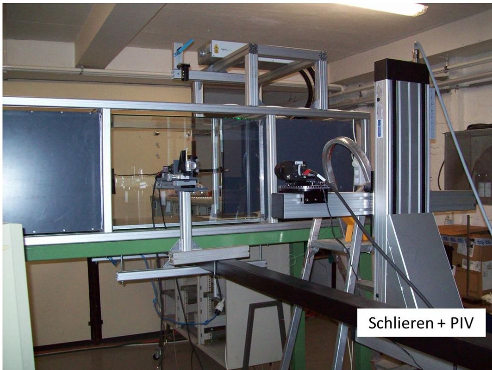
Figure 3. The measurement setup [own photo]
