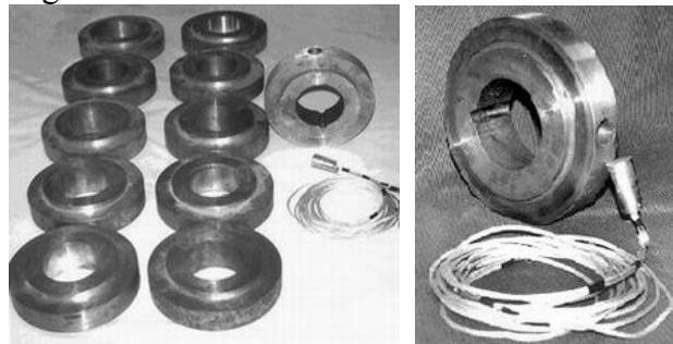
Figure 2 Assembly of conical pin fitted Pt-Pt/RH thermocouplings
