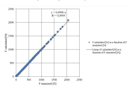
Fig. 11. Relationship between the measured force and calculated force using (16)
