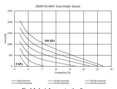
Fig. 4. Isobaric force-contraction diagram
