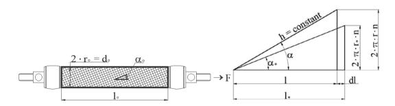
Fig. 2. Geometry parameters of PAMs
