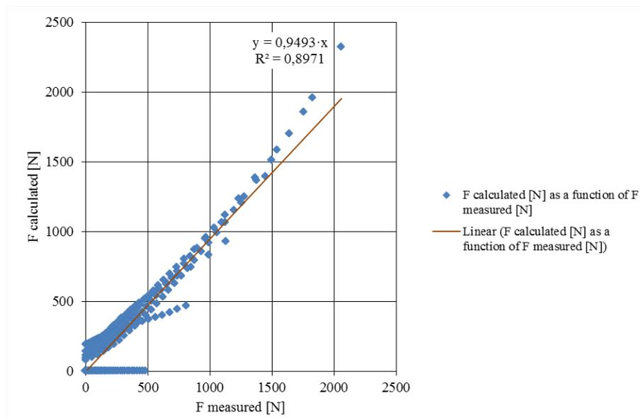
**Fig. 8. Relationship between the measured force and calculated force using (15)**
